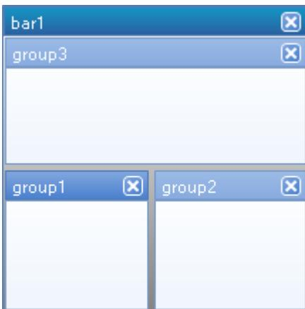
**ToolWindow** - This appearance emulates the docking functionality of Visual Studio .NET. All Groups are visible and have headers. Windows can be docked anywhere in the container and can be represented by tabs with four types of orientation.
